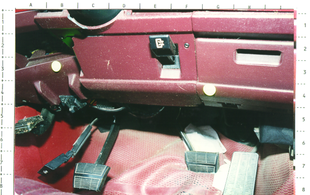
# 82 -- Close-up of contacts to 1988 Chevrolet pickup's lower dash from driver's knees; NOTE: entrapment occurred in toepan area
